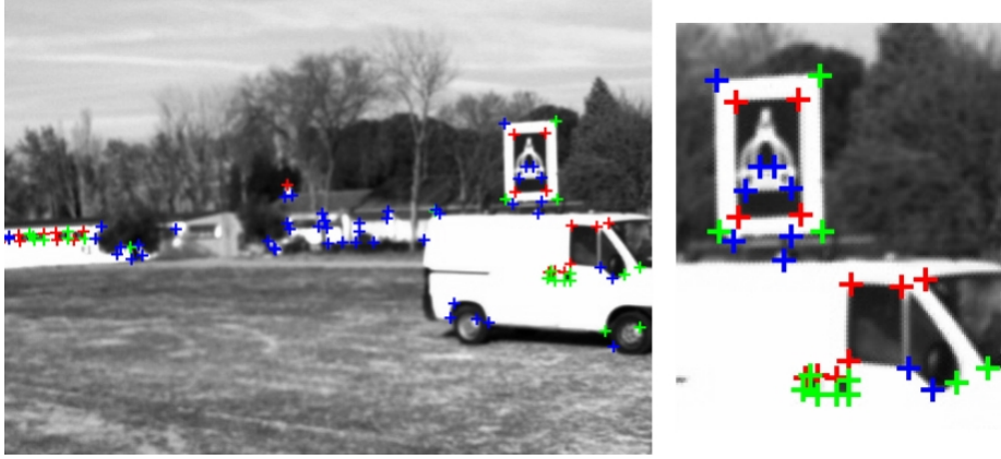
Fig. 2 Extracted corners features classified into three levels. Red corners are the most stable ones and belong to level 1 group. Green corners are classified as level 2 and blue ones as level 3.
