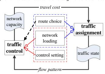
Figure 1: Interaction between traffic assignment and traffic control
