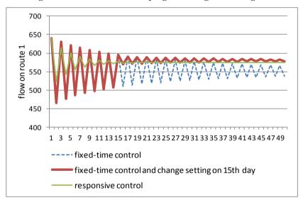
Figure 5: Effect of a fixed-day signal setting on convergence
