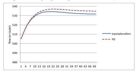
Figure 3: Flow trajectory under equisaturation control and P<sub>0</sub> control
