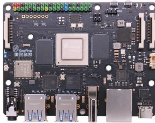
Figure 6.4: StarFive VisionFive2 RISC-V board (SiFive U74).
