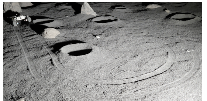
Fig. 4: Real-world validation is performed with a Leo Rover inside the LunaLab facility [25], which serves as a lunar-analogue testbed filled with basalt gravel. It is equipped with a Sun emulator and a motion capture system for ground-truth state estimation during policy execution and evaluation.
