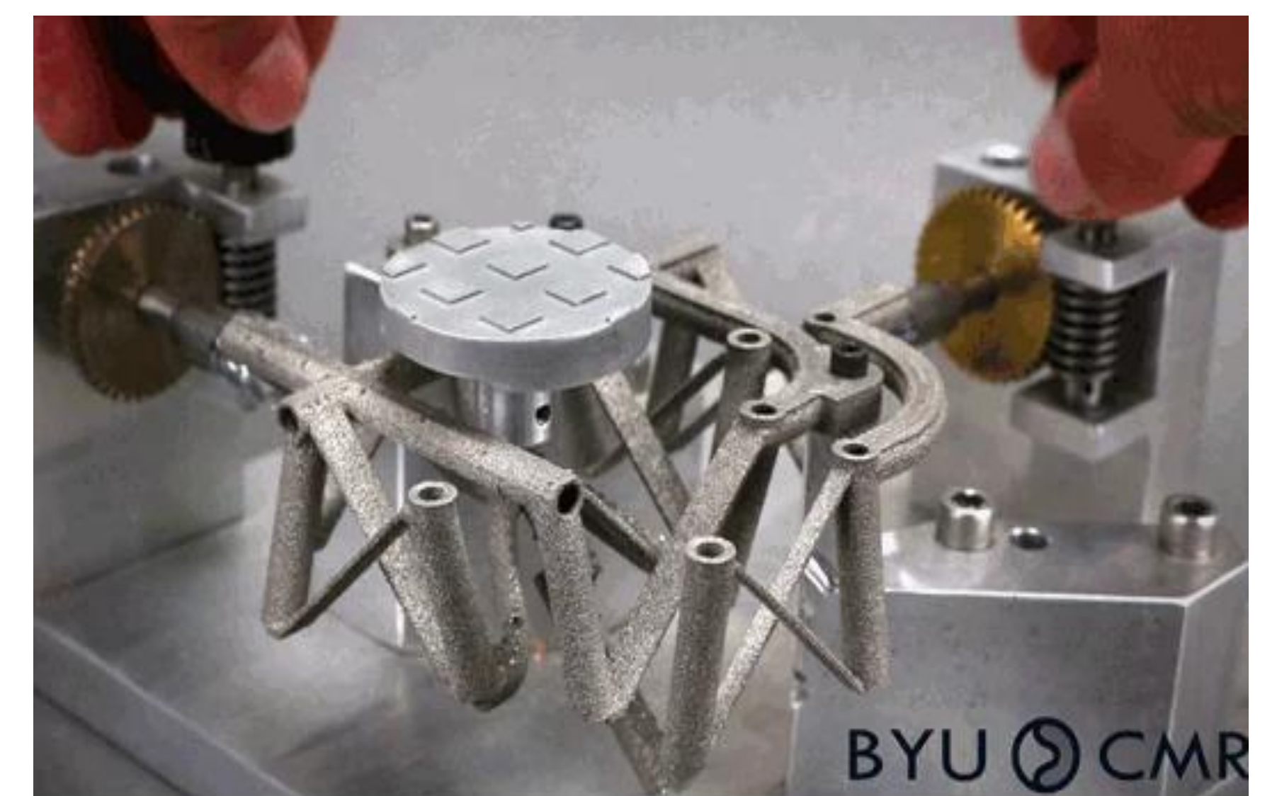
Monolithic 2 DOF fully compliant space pointing mechanism by E.G. Merriam et al.
