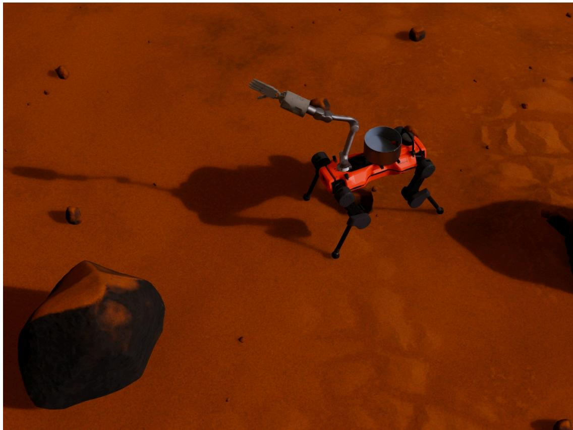
**Figure 4.2** – An example of the modular composition of robots in SRB. The framework allows for the combination of any compatible mobile base with any manipulator and EE to create novel mobile manipulation systems.
