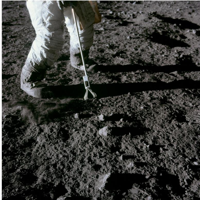
**Figure 2.1** – A photograph of the Apollo 12 mission displaying the use of a manual tool for collecting lunar rock samples [42].
