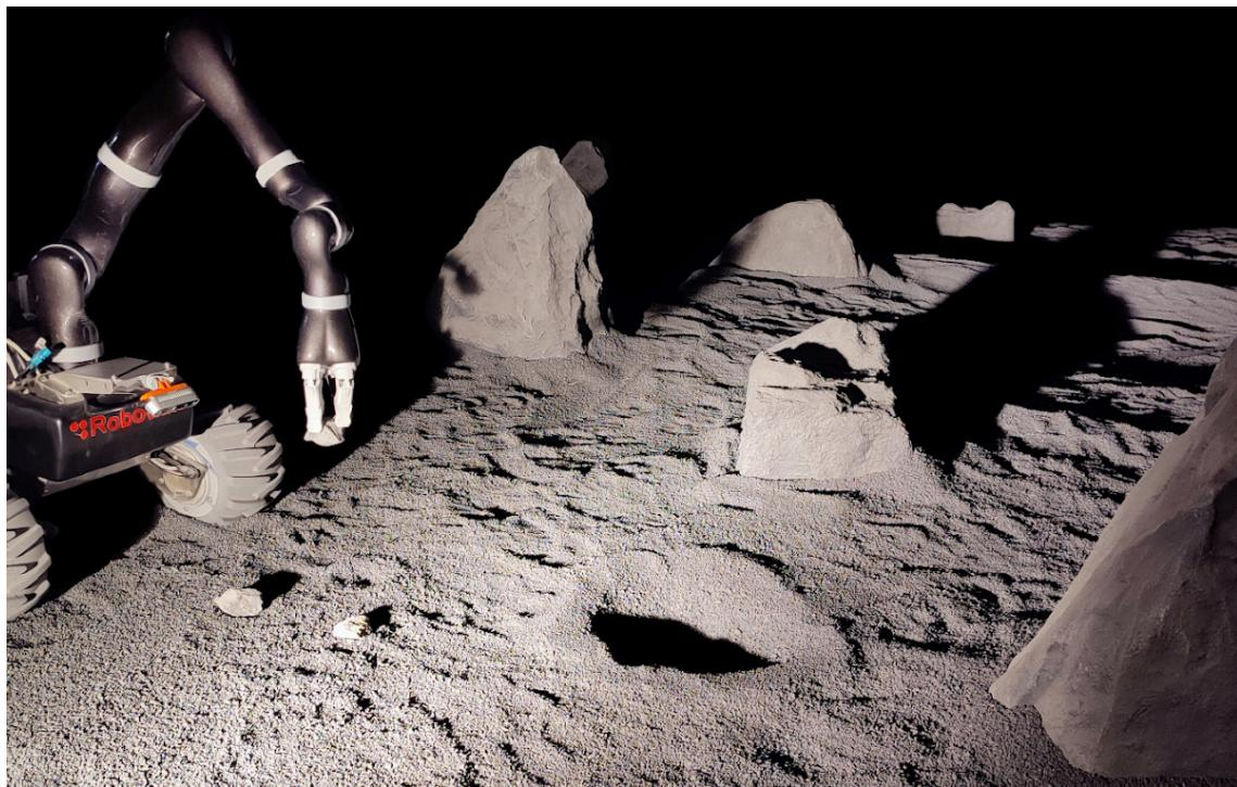
**Figure 3.7** – The physical setup for the sim-to-real validation experiments, conducted in the LunaLab facility at the University of Luxembourg that is filled with 20 tons of basalt gravel [37].
