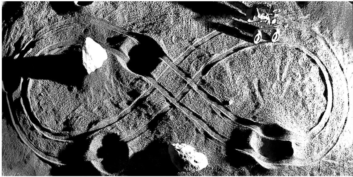
**Figure 6.8** – Repeatable lemniscate path imprinted by the rover’s wheels in the basalt gravel of the LunaLab during a real-world deployment.
