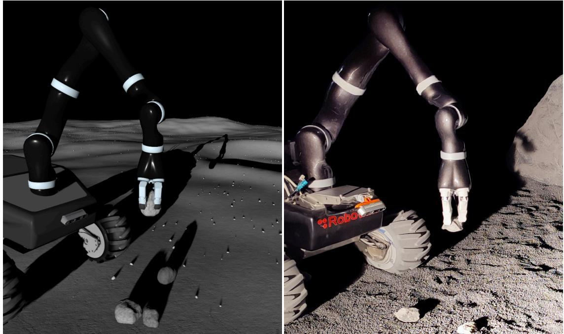
**Figure 2.8** – A conceptual illustration of the sim-to-real gap, taken from the foundational study of Publication I. A policy trained exclusively in a simulation domain may fail when deployed in the real world due to discrepancies in physics, visuals, and other unmodeled effects.
