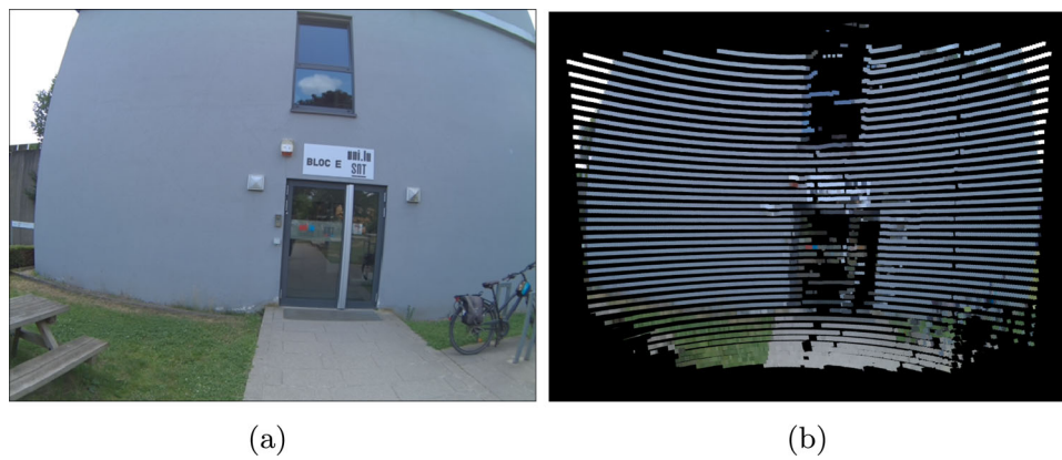
Fig. 3 Qualitative calibration validation using point cloud colorization with the front-right camera. (a) raw camera image; (b) LiDAR point cloud colored by the projected image. While the alignment is generally consistent, minor misalignments are visible at building edges, reflecting residual calibration errors
