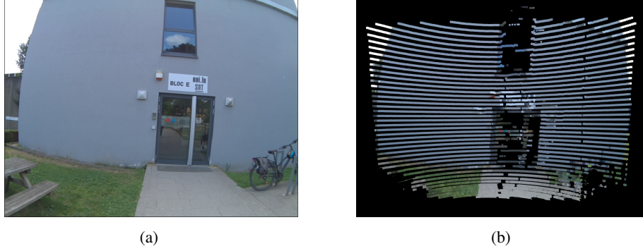
Figure 3: Qualitative calibration validation using point cloud colorization with the front-right camera. (a) raw camera image; (b) LiDAR point cloud colored by the projected image. While the alignment is generally consistent, minor misalignments are visible at building edges, reflecting residual calibration errors.
