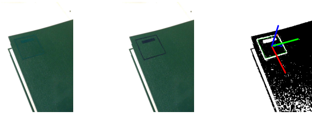
(a) Static single-vision setup detecting a visible-range iMarker: raw frame (left), polarizer applied (middle), and detection result using color masking (right).
