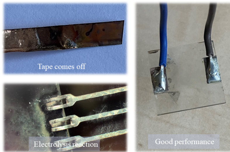
FIG. 4.6: Wire connection power test results
