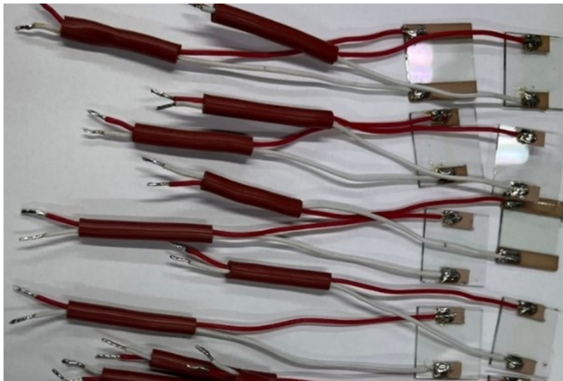
FIG. 4.7: Final ITO sample prepared via silver-paste sintering and soldering.
