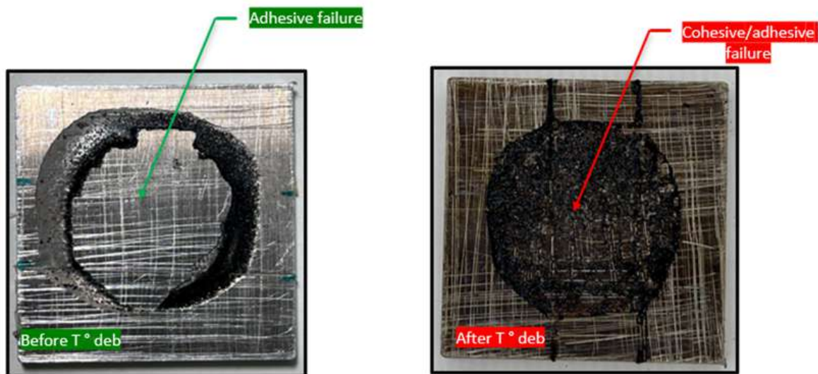
Figure 5.4: Observation of disjointed substrates before and after debonding.
