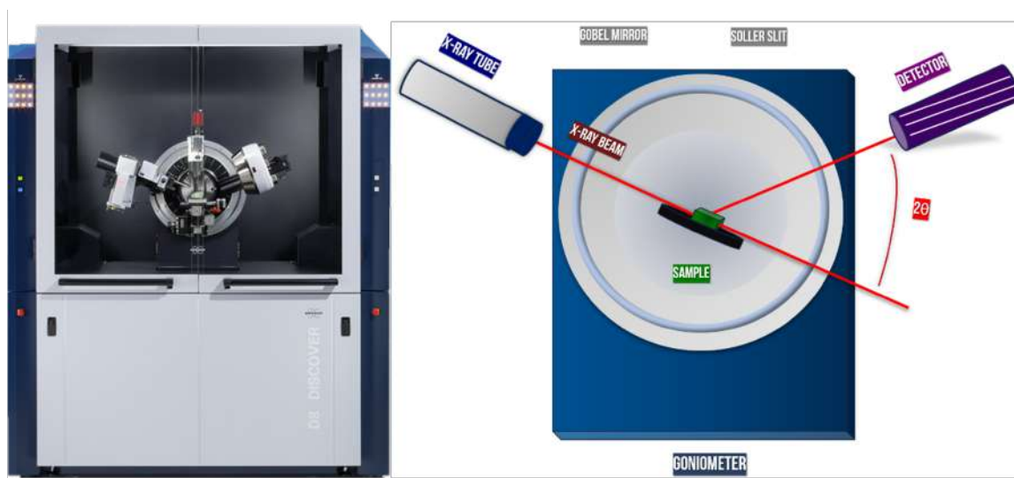
Figure 2.17: Schematic representation of X-Ray diffraction experimental set-up and the a Bruker D8 Advance diffractometer instrument.
