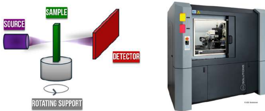
Figure 2.15: Schematic representation of tCT experimental set-up and the EasyTom 160 micro-CT instrument.
