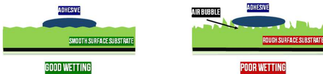
Figure 1.7: Schematic representation of the wetting theory.
