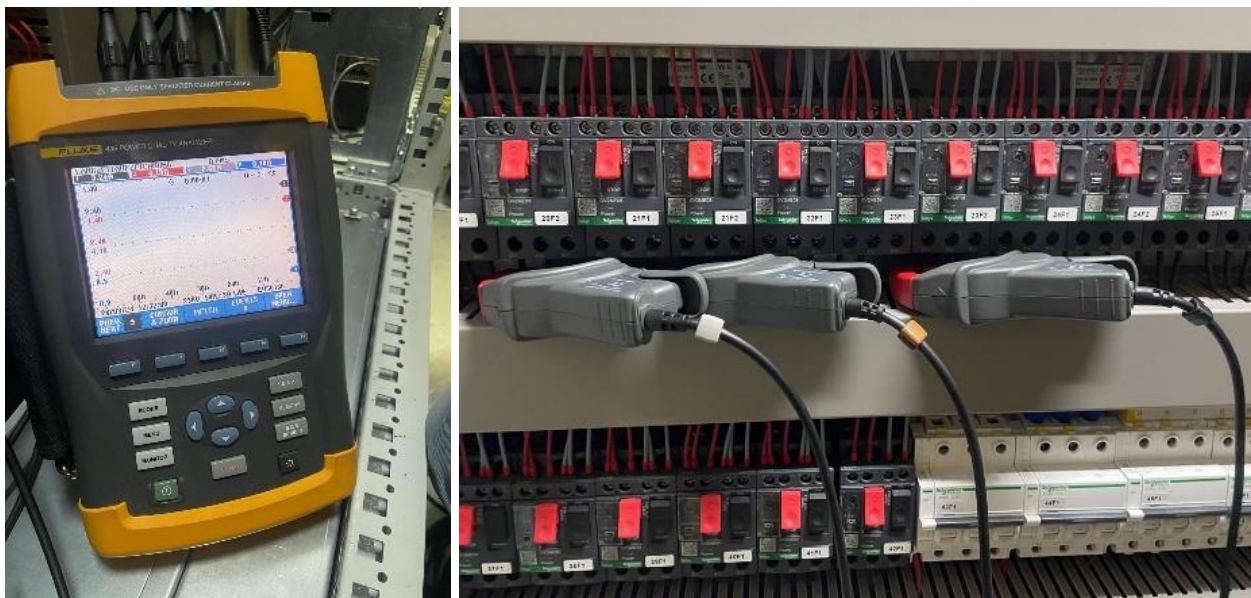
Figure A.2: (a) Electrical meter; (b) Current clamps
