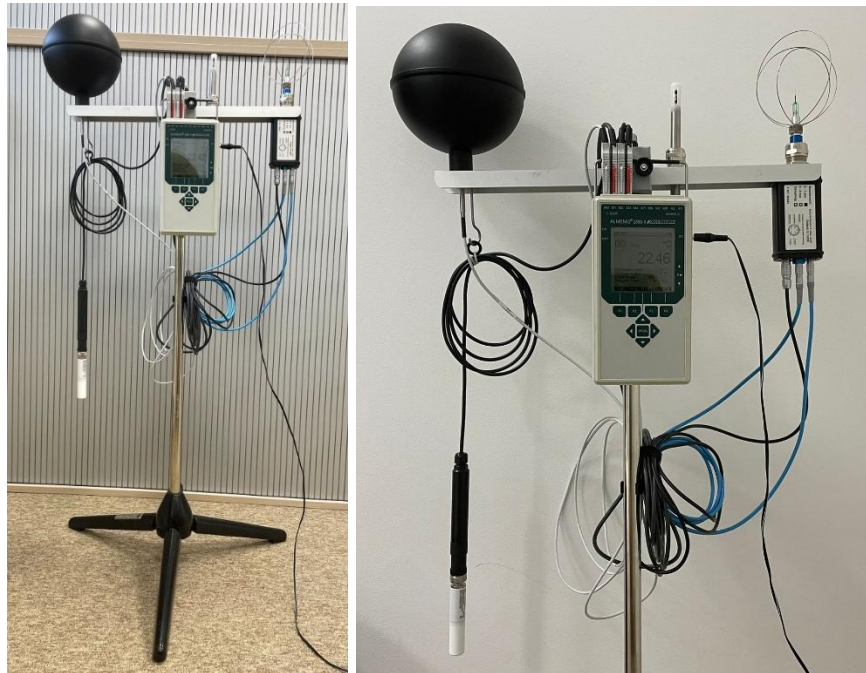
Figure A.4: Thermal comfort sensors (a) setup showing height (b) setup sensors detail
