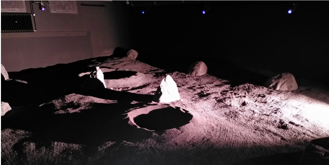
Figure 3.7: LunaLab, University of Luxembourg. Equipped with an illumination system simulating lunar south pole lighting conditions.
