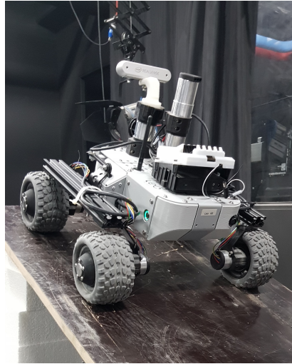
Figure 3.6: Experiment to determine the maximum slope inclination the rovers can traverse
