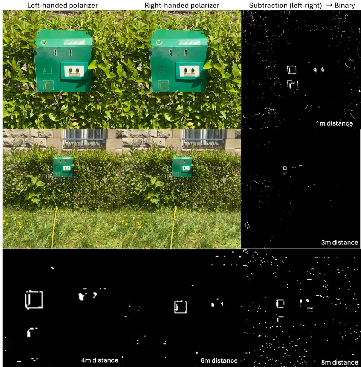
Figure 4.17: Comparison of long-range visibility of a G-d-CSR-marker, G-CSR-marker and two jewel beetles in an outdoor scene using a mobile phone-based time-sequential dual-polarization imaging setup. Images were captured through left-handed and right-handed circular polarizers at increasing distances. The top two rows show the LH, RH, and subtraction images, at 1m and 3m. The bottom rows display only the subtraction images (zoomed-in versions) at 4m, 6m, and 8m distances.
