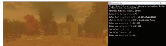
Figure 12: External VE control via example Python console application controlling a visual stimulus (golden flashing).
