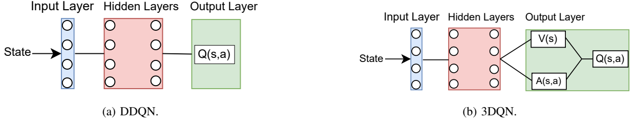
Fig. 5: Q-value estimation process in DDQN and 3DQN as in [48].
