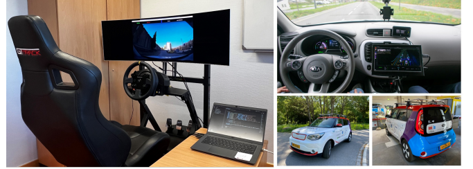
Fig. 1: Experimental vehicle based on Kia Soul EV with the teleoperated driving interface.
