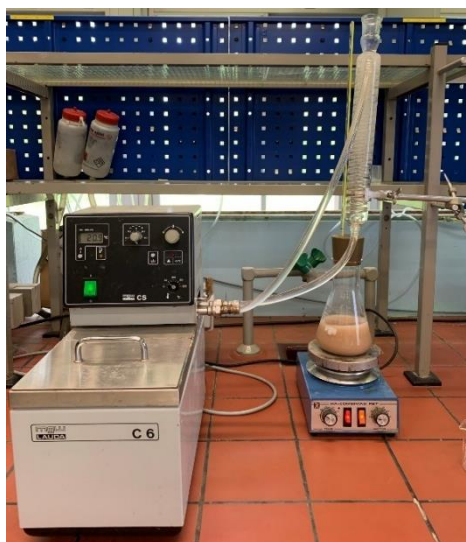
Figure 35. Chapelle test setup in the laboratory.
