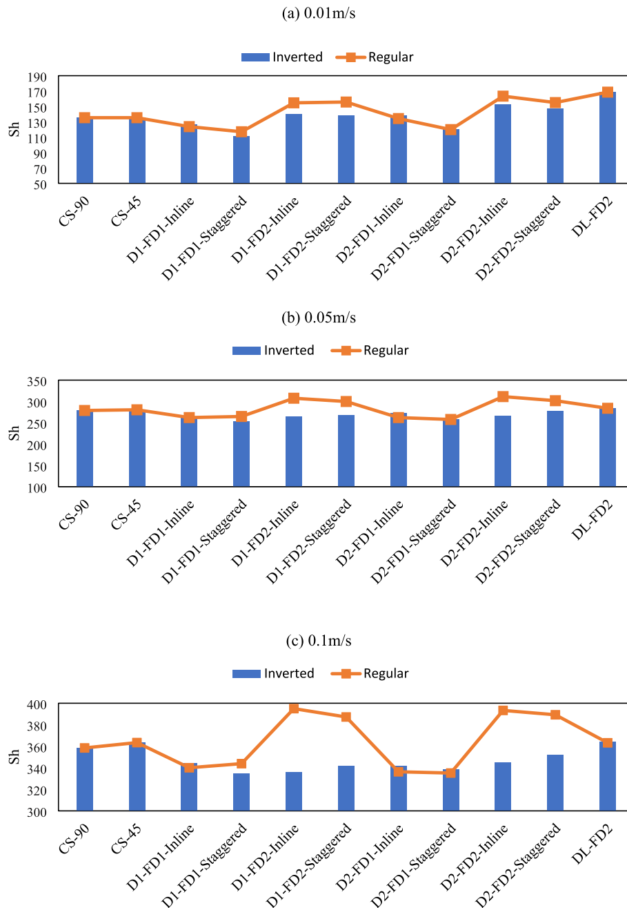
Fig. 23. Sherwood number ( Sh ) values for all proposed spacer configurations compared CS-90 and CS-45, analyzed in both the regular and inverted scenarios, across the velocity range studied.
