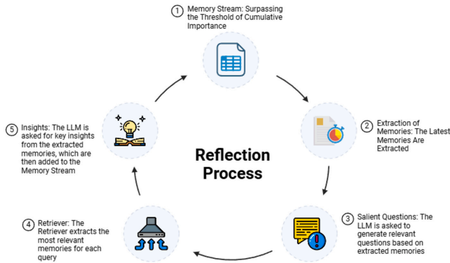
Fig. 4. Reflection Mechanism Process: 1. An accumulated threshold of importance is reached, 2. The most recent memories are extracted, 3. The LLM is asked for the most relevant questions based on the memories, 4. Using the Retriever, the most relevant memories are extracted for each question, 5. Insights are generated from the extracted memories and are then stored in the Memory Stream.
