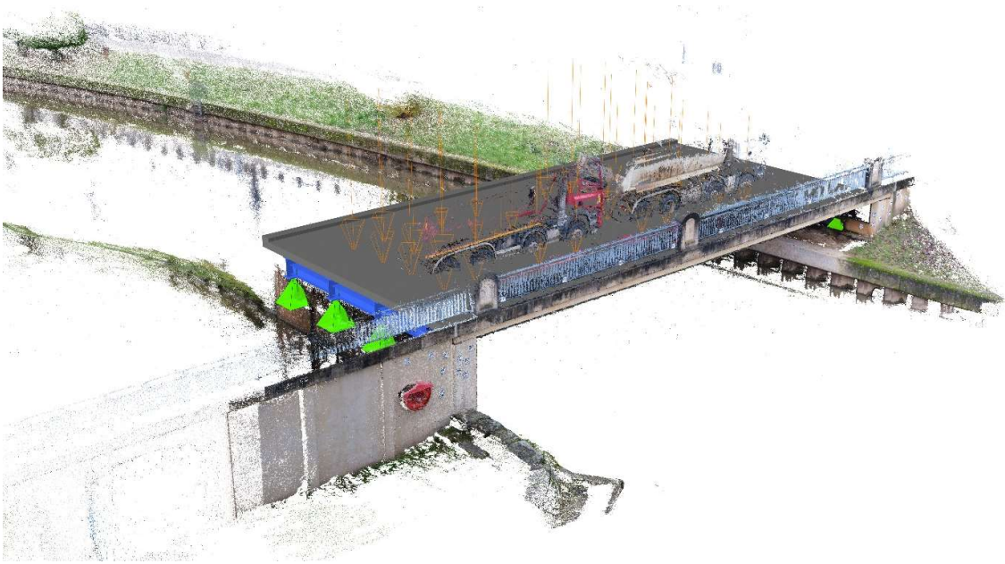
Figure 90. Point cloud overlayed with the structural model to validate geometry and calibrate loading positions
