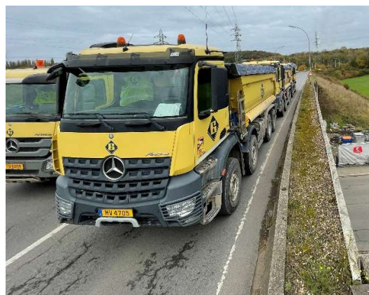
Figure 84. Heavy trucks serve as loading for the Soleuvre bridge experiment
