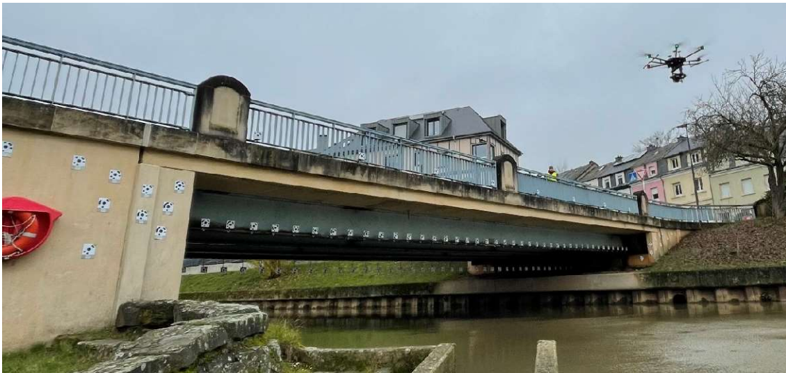
Figure 87. Image Acquisition of the unloaded state of the Ettelbrück bridge
