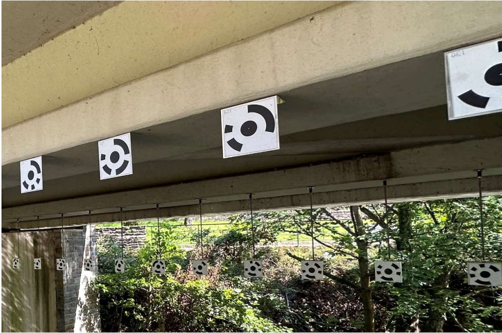
Figure 58. Photogrammetric targets attached on outer and middle girder with bolts
