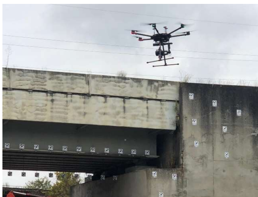
Figure 83. Image acquisition using a UAV Soleuvre bridge; unloaded state
