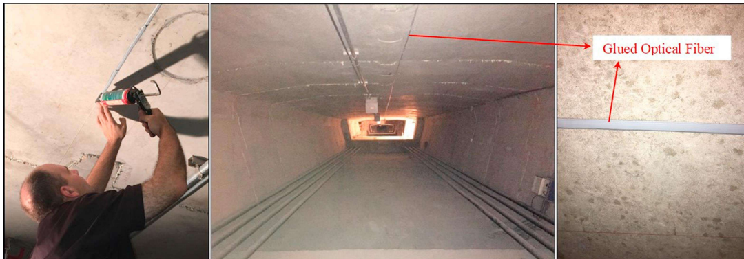
Figure 9. Optical fiber for strain measurement of a bridge structure [88]
