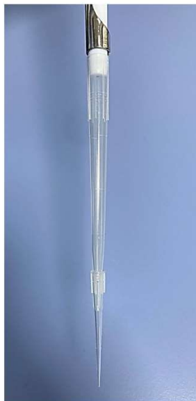
Figure 4. Double plastic tip to enhance MMS dissociation
