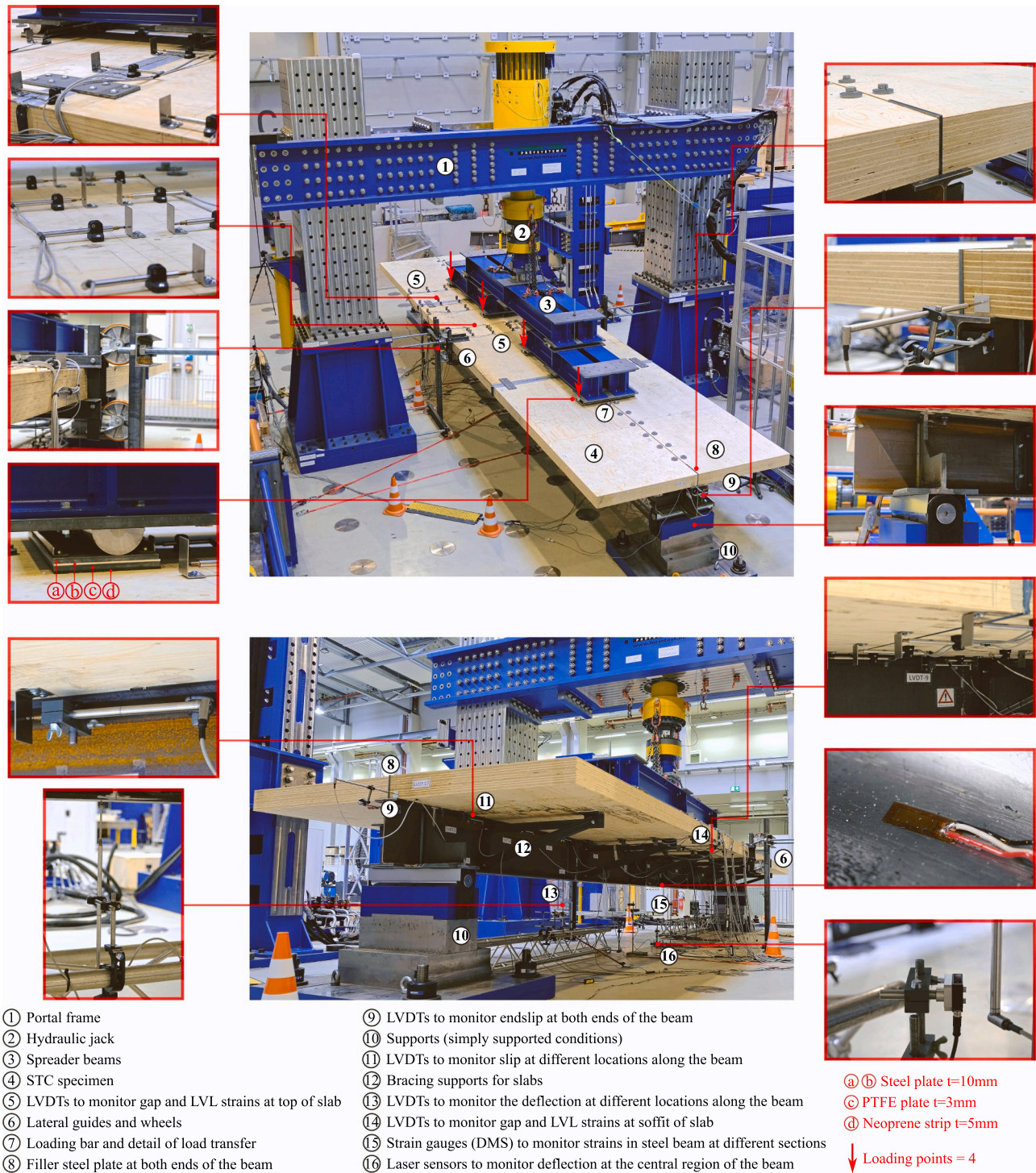
Fig. 10. Test setup and instrumentation of the STC beams.
