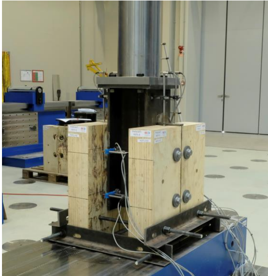
Figure 12: Push-out test setup.
