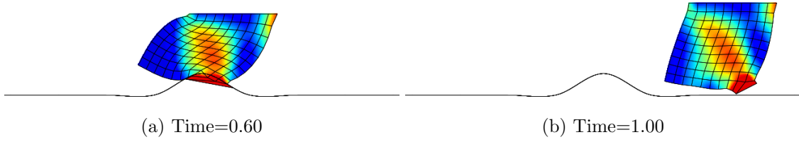
Figure 2.25: 2D hyperelastoplasticity, 10 \times 10 FEs. Two deformations predicted by the TR methods.
