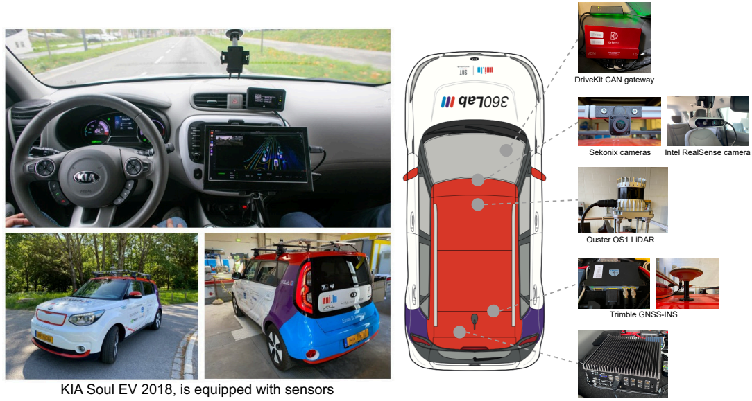
FIGURE 2.2: Demonstration of the sensor configuration employed in the autonomous vehicle at 36Lab, SnT, University of Luxembourg. The setup includes a LiDAR for 360-degree environmental mapping, multiple cameras for visual data acquisition, and a GNSS-INS for high-precision localization. Source: Adapted from [142], with permission.
