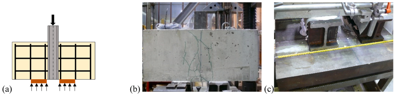
Fig. 11. Experimental set-up for push-out tests (a) schematic diagram and (b) test set-up and (c) supports.
