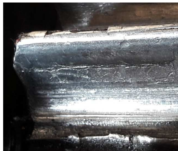
Figure 11. Surface of the tooth - abrasive and fatigue wear.
