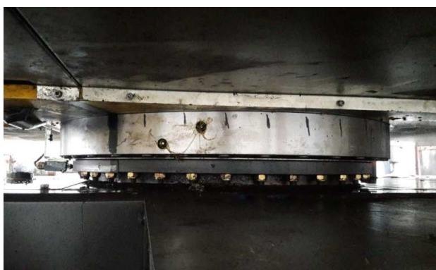
Figure 6. Mounted slewing bearing.
