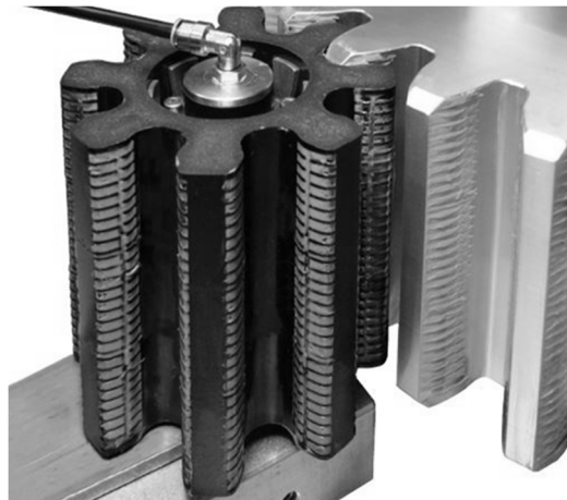
Figure 16. Polyurethane (PU) lubrication pinion [6, 7].
