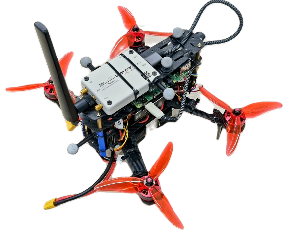
Fig. 2. UAV equipped with USRP and Raspberry Pi used for the experiments.
