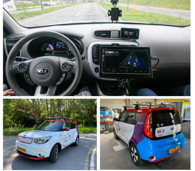
Fig. 1: The experimental vehicle based on a 2018 KIA Soul EV retrofitted with hardware and sensors enabling self-driving operation.
