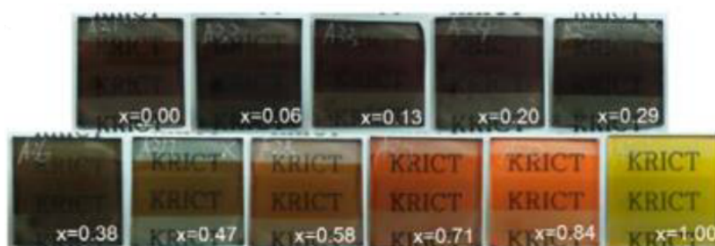
Figure 2.3: Sequence of pictures of \text{MAPb}(\text{I}_x\text{Br}_{1-x})_3 for different x values from x = 0 to x = 1 . Figure taken from [26].
