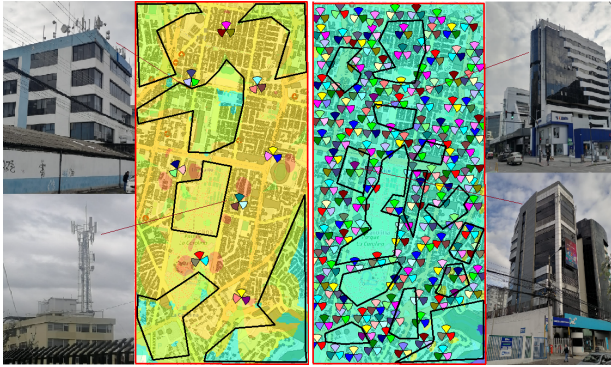
Fig. 7. Dead/shadow zones 3.5 GHz (left) and 28 GHz (right).
