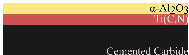
Figure 2.2: An overview of the material produced. A multilayer coating of \text{Ti}(\text{C,N})/\alpha\text{-Al}_2\text{O}_3 is deposited on a cemented carbide substrate using a two-step coating process.
