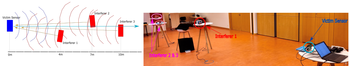
Figure 2.8: Details of the arrangement of the victim and interferer sensors along with the picture of actual measurement setup.
