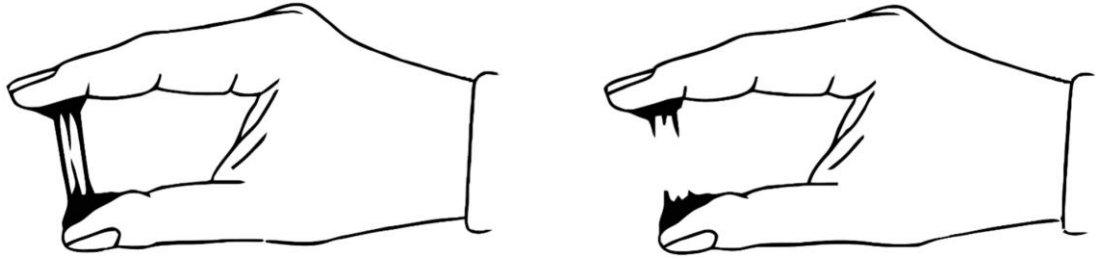
Figure 6: Tack and stringiness assessment using the finger test [51].
