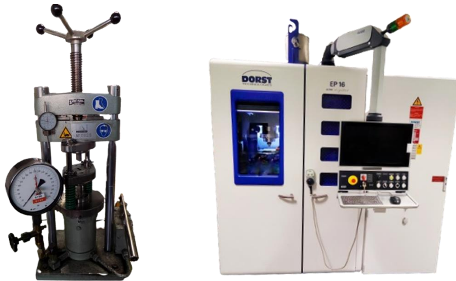
Figure 22: (left) Manual hydraulic and (right) DORST TECHNOLOGIES EP16 used for the development of the methodology to assess the CBVC_{P0} with the uniaxial die method developed in this study.
