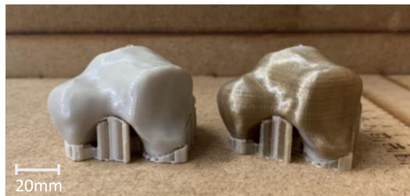
Figure 13. PEEK talus after the heat treatment (left) and before (right).
