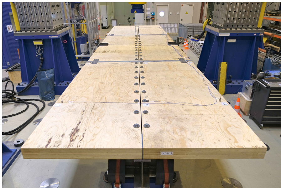
Figure 9.2: Instrumentation of the STC beam with accelerometers for the vibration test.
