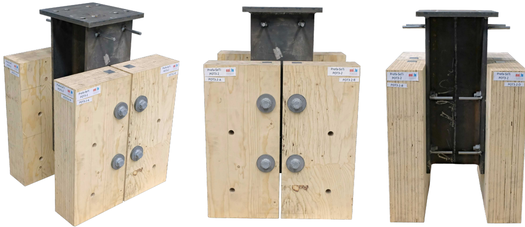
Figure 5.6: Pictures of a push-out test specimen.
