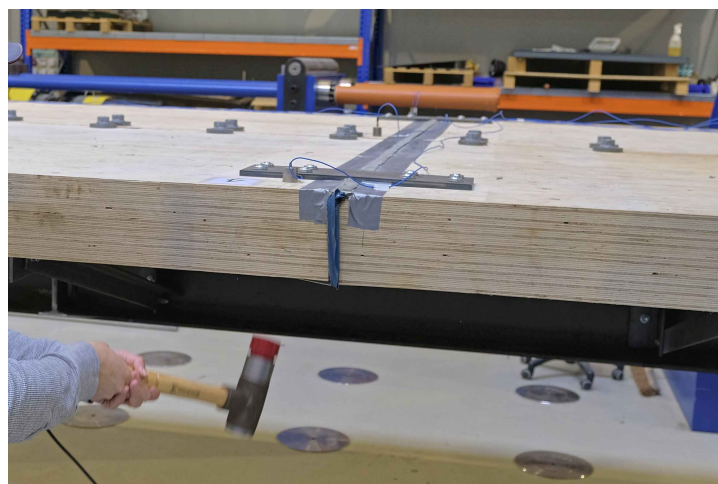
Figure 9.4: Excitation with hammer hit at the soffit of the LVL slab.
