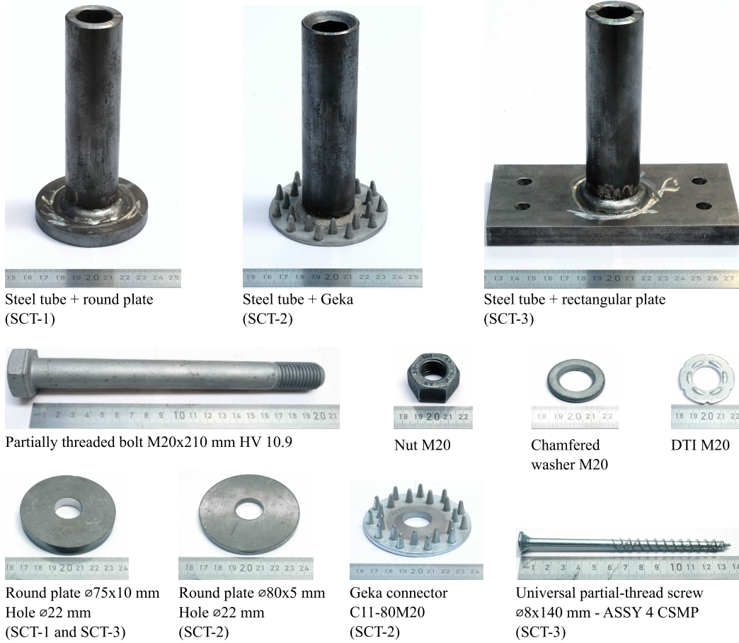
Figure 5.2: Components of the shear connections.
