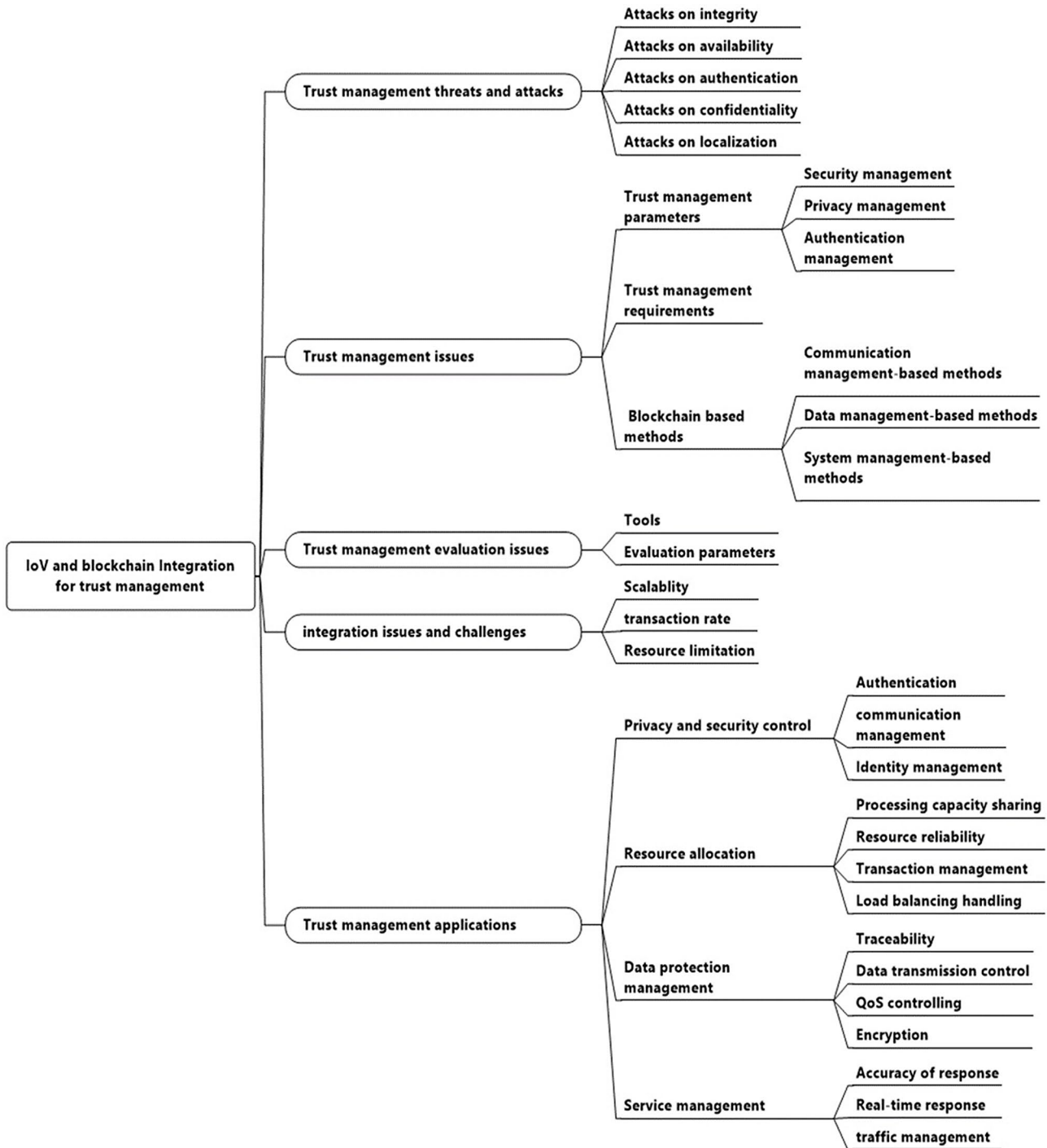
Fig. 3 A proposed taxonomy for Integration of IoV and blockchain for trust management
