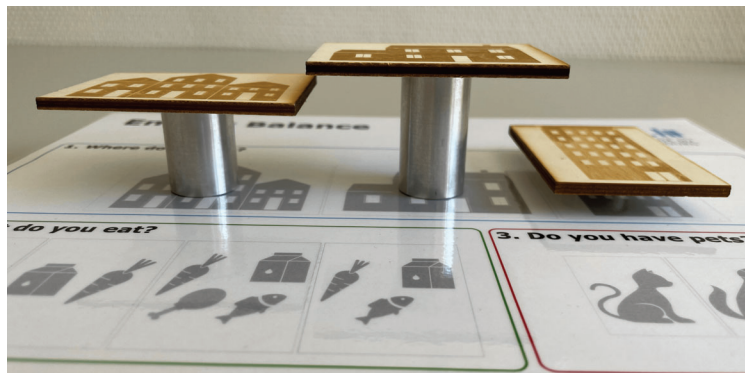
Figure 6.4: Side view of three answer tokens with different areas, heights and weights.
