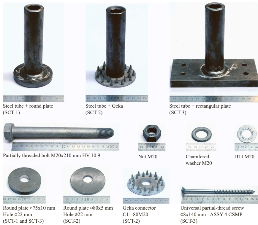
Fig. 2. Pictures of the components of the shear connections.
