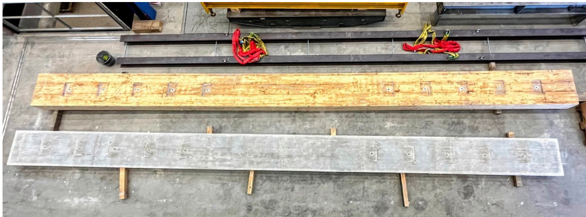
Figure 30. Demounted CCC-B2 slab after failure.
