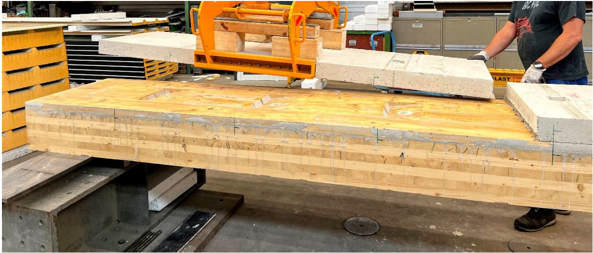
Figure 31. Demounting concrete slab from CCC-B1 after the first loading cycle.
