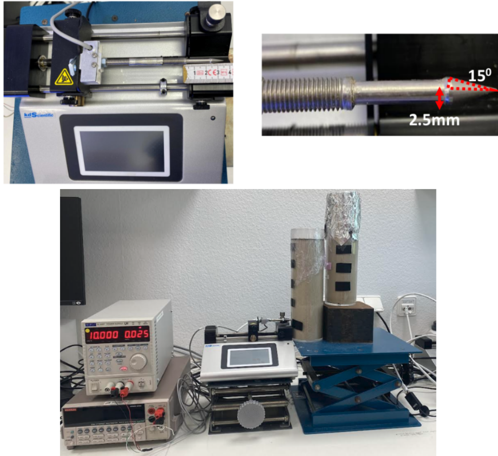
Figure 2.1: (Above) Penetrometer needle dimensions and (Below) Full penetrometer set-up.
