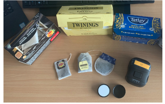
Fig. 7: The teabags and NIR spectrometer used in our experiments.
