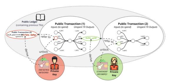
Figure 2: anatomy of a transaction in a UTXO-based system From: Pocher N, Zichichi M, Ferretti S (2023)
