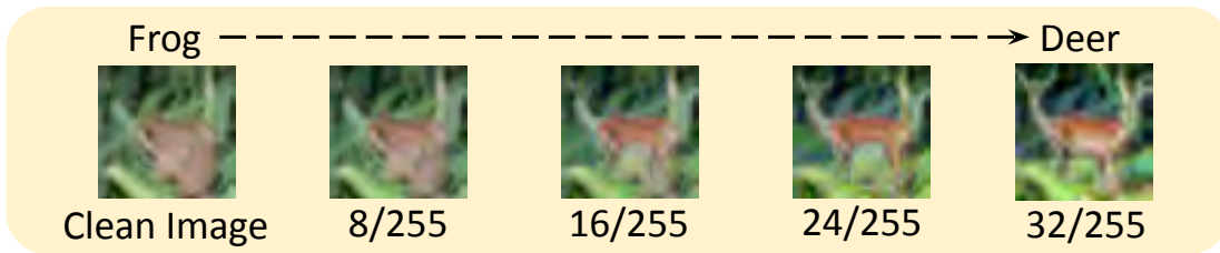
Figure 1.2: Large perturbations may be visible and can even change the label. Illustration from Addepalli et al. [AJS + 22] of an original image of a frog altered to the deer class with increasing \varepsilon , the L_\infty norm of the perturbation. The frog looks partially like a deer at \varepsilon = 16/255 , which is the norm widely used to evaluate transferability.
