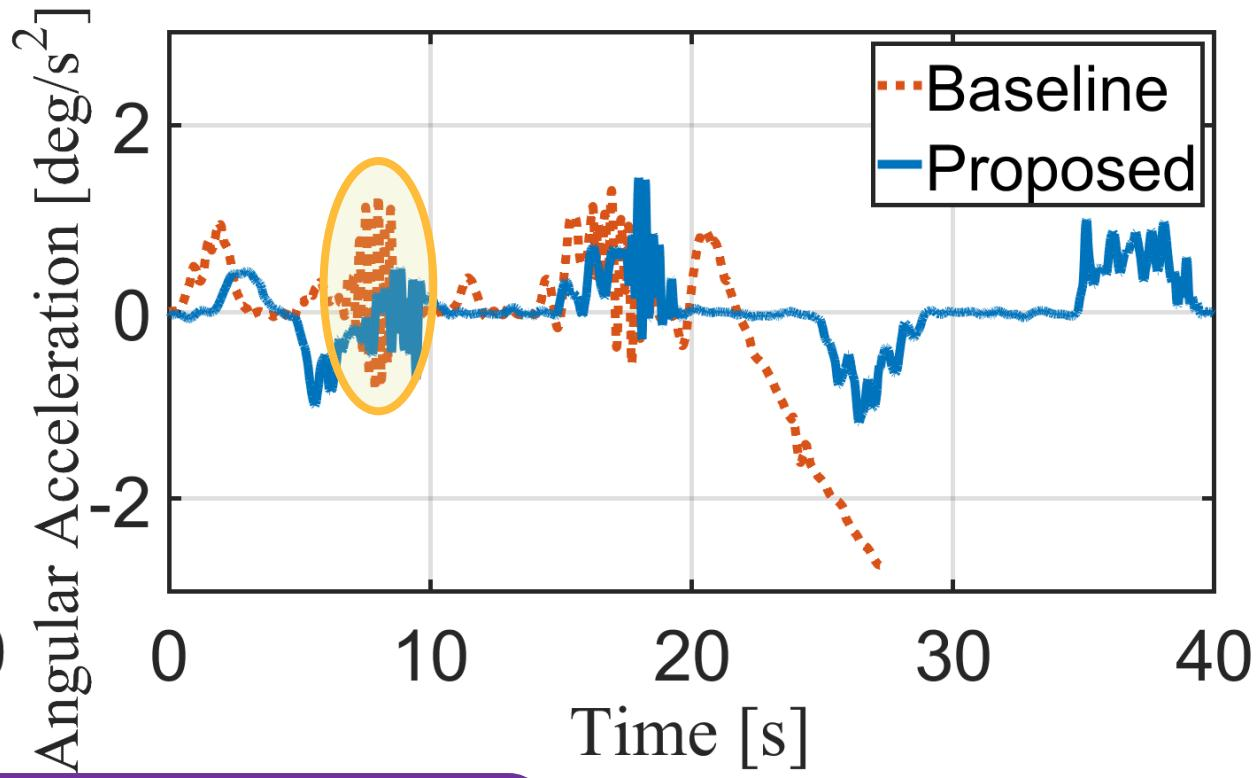
Proposed method **reduces max. acceleration** during swinging phase, increasing locomotion stability
