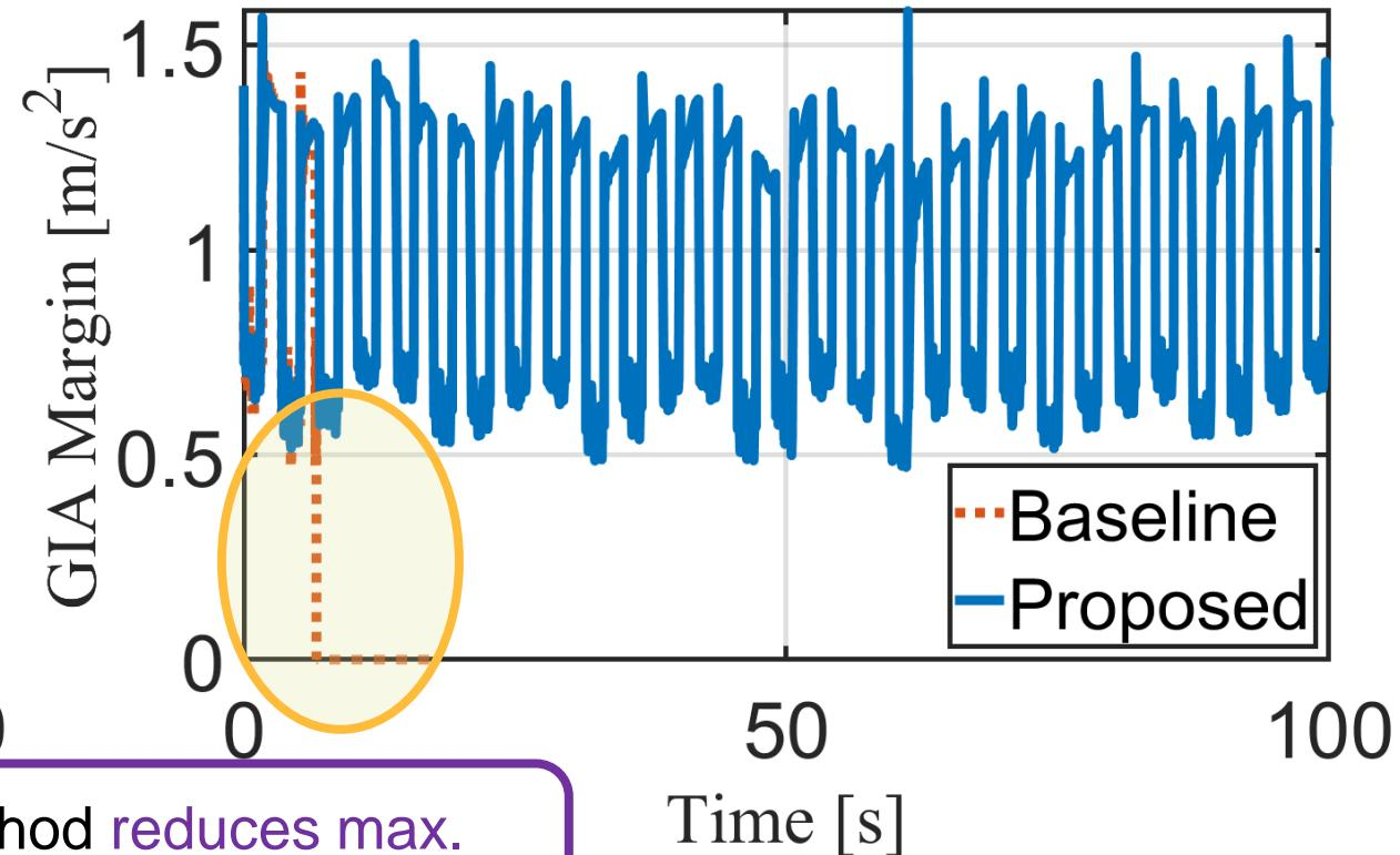
Proposed method reduces max. contact forces, increasing stability
