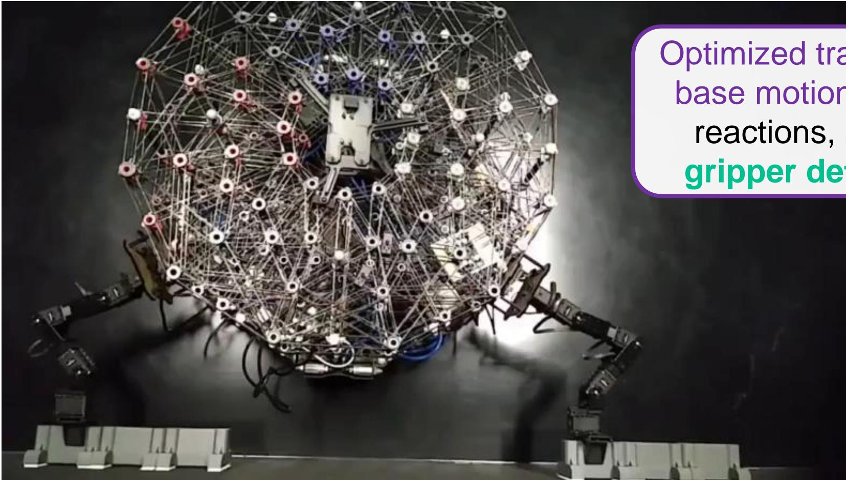
Optimized trajectory and base motion to reduce reactions, **avoiding gripper detachment**
