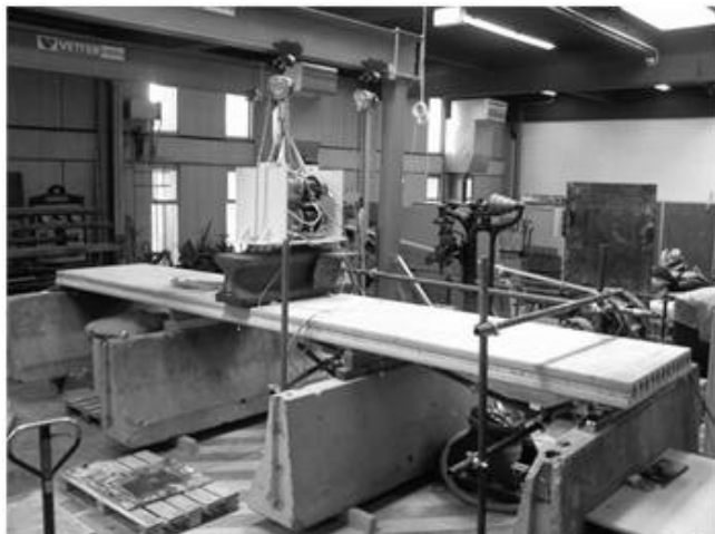
Figure 5. Experimental setup for the static testing for the first test series with an unbalanced special mass exciter.
