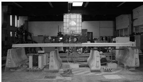
Figure 7. Experimental setup for the static testing for the third test series with the three steel weights and the water tank.
