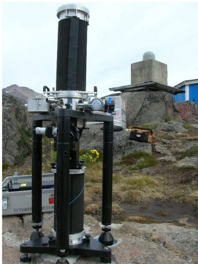
FIGURE 1 FG5-216 absolute gravimeter at the gravity site of Kulusuk, southeast Greenland. The permanent GNSS antenna is visible in the background. The blue shed is equipped with electric power and hosts the GNSS receiver.
