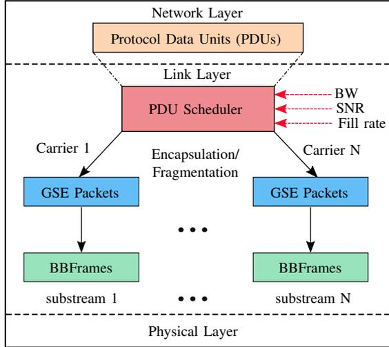
Fig. 2. The protocol stack of carrier aggregation.
