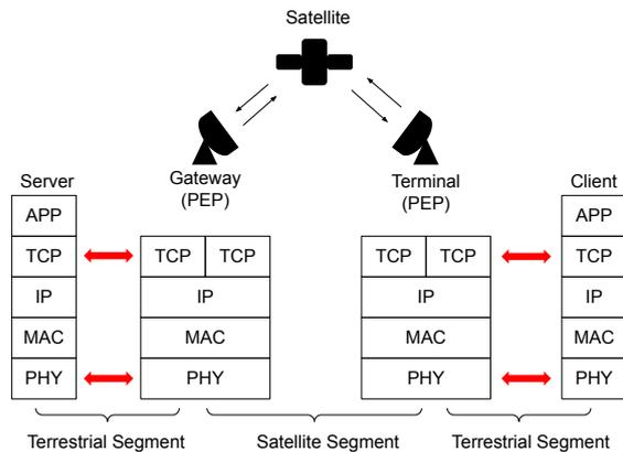
Fig. 4. PEP based TCP splitting for satellite links
