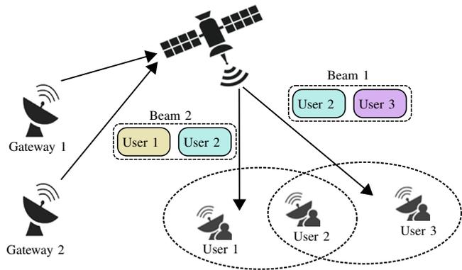
Fig. 1. Schematic diagram of inter-beam carrier aggregation in a multi-beam satellite system.
