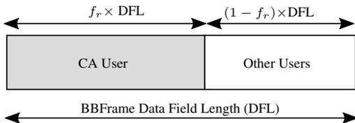
Fig. 3. Fill rate illustration in the BBFrame structure.
