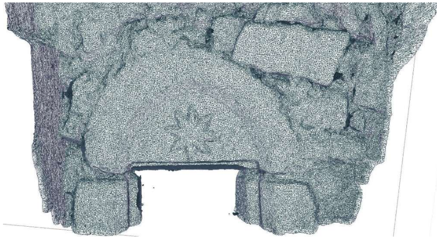
Figure 6 - an example of a high-LoD relict element, a photogrammetric model of a surviving door in the Criechinger Haus
